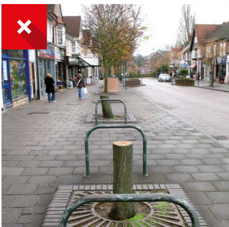
Insufficient rooting volume - after a good start these trees exhausted available soil.
