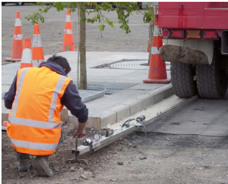
The RootCell structure underneath this pavement was subjected to 400 passes of an 8.2 tonne (9 ton) axle loading immediately adjacent to the structure and then a further 200 passes immediately above the RootCell . As expected, no adverse movement of the structure was detected
