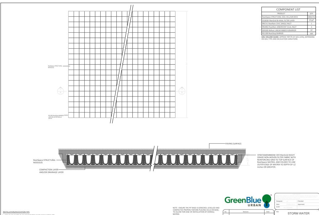
1. ADD 5% TO OUTER PLAN DIMENSIONS WHEN EXCAVATING PIT. 2. ALWAYS CHECK PIT DIMENSIONS AT BASE OF PIT, ENSURING SIDES ARE CLEAN AND SQUARE
