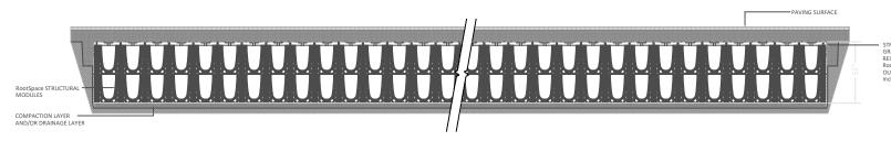
STRATAMEMBRANE OR FilterGrid HEAVY GRADE NON-WOVEN FILTER FABRIC WITH REINFORCING GRID TO TOP SURFACE OF ROOTSPACE MATRIX, AND FOLDED TO LINE OUTER EDGE OF MATRIX TO DEPTH OF 12 inches OR GREATER.
